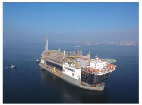
Largest ever cargo transported by a Heavy Transport Vessel at 80,000 MT and 288m length
